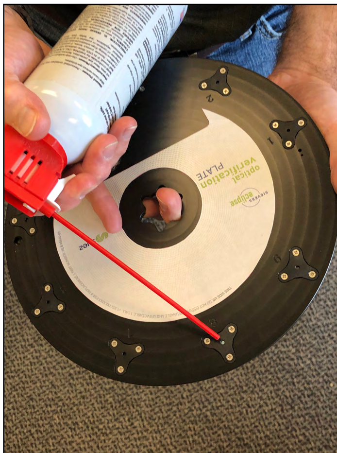
Figure 7-3: Using compressed air to clean OVP filters
